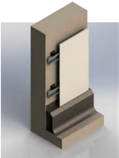
05. Waterproof footing of wall with hanging panel
